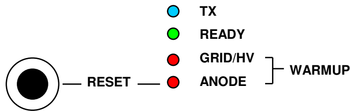
Figure 7: A front-panel layout for the LED array and RESET button.
